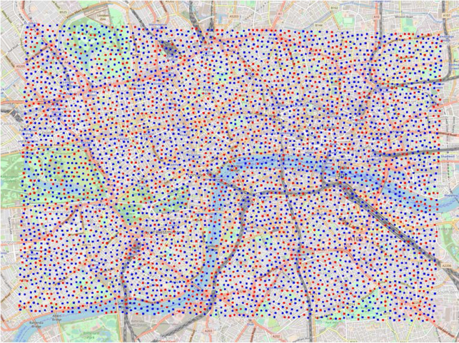
Fig. 8. LAEI cells sampled for the experiments. The 3,000 blue cells are the training data set and the 1,500 red cells are the test data set. (Underlying OpenStreetMap Image: ©OpenStreetMap contributors).
